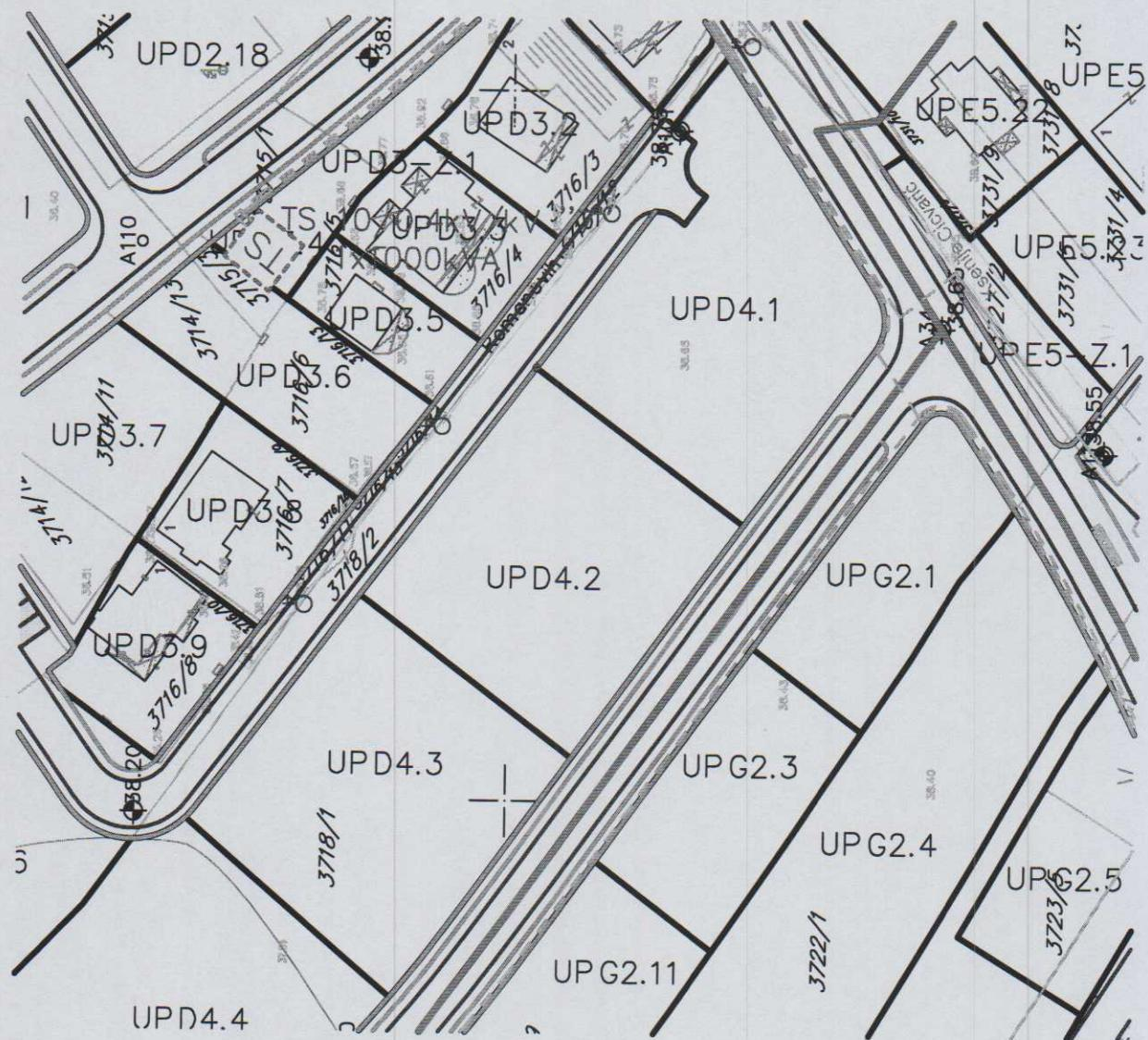
Planski trafo reon 10, planirana trafostanica TS TS 10/0.4kV/kV "7", 1x1000kVA
